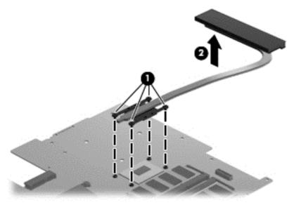
**d.** Thoroughly clean the thermal connections (1) on the system board and the heat sink (2) before replacing a heat sink onto a system board.
